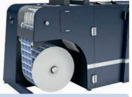
Eg. 8-up labels on A4 sheet ▶ capable to print 10,000 labels(263m) in approx. 25min(13.5m/min).
