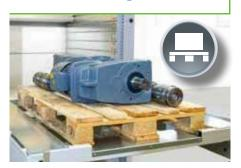
The "pallet handling" application ensures that pallets can be placed directly on the pallet trays by means of forklift or pallet truck and stored in the positioning facility. This saves floor space and reduces the need for high-rack stacker trucks. In addition, stored goods are found much more quickly. In summary, this application effectively helps to cut costs and raise productivity, and is also a plus from a safety perspective.
