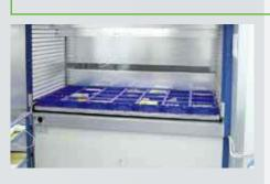
The extractor device delivers the requested tray to the access opening or back to a free storage location within the device at fast speeds. At the push of a button or scan of a barcode.
