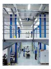
Vertical lift modules can go through several floors with up to six access openings placed on the front or rear side of the unit. A mezzanine floor can be installed to enable operation on several levels at the same time (with loading at one level or side and retrieval at the other).
