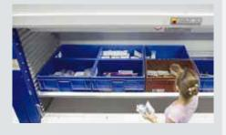
Side walls of the access opening are equipped with L-profiles. These enable the positioning of multiple trays in the access opening (double-access handling) as well as individually adjusted working positions for each operator depending on their physical height.
