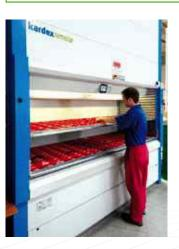
Thanks to the double-access handling option it is possible to use two work levels in the access opening. A tray is transported into the first work level in the access opening and the shutter door closed. While articles are stored or removed, the next tray is being retrieved and kept in a waiting position behind the access opening.
